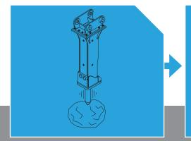
When the breaker operates in normal conditions the tool is in contact with the rock and strikes.
